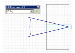
Figure 6A-4A: The **Centerline Style** horizontal line, the inclined line and the **Mirror** tool.
