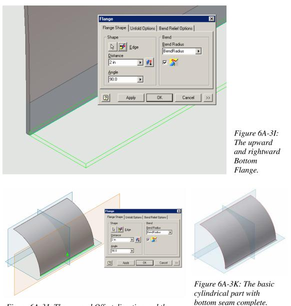
*Figure 6A-3J: The upward Offset direction and the rightward Flip Direction.*
