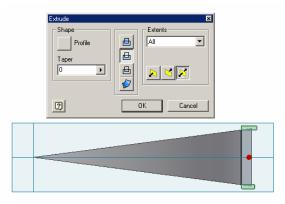
Figure 6A-5D: Cutting off the inclined ends with the *Extrude* tool.
