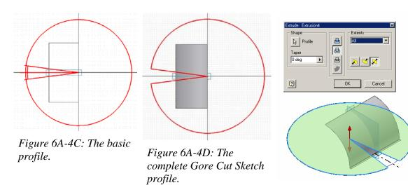
Figure 6A-4E: Cutting the semi- Gore segment.
