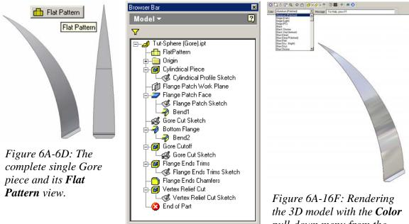
Figure 6A-6E: The features listed in the Model panel.
