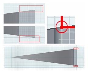
*Figure 6A-5C: The rectangular cutoff profiles.*
