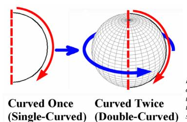
Figure 6A-1A: The "curved once" semi-circular profile used to generate a "curved twice" or "double-curved surface of a sphere.
