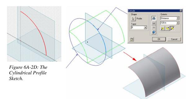
Figure 6A-2E: The Cylindrical Piece Extrude feature .
