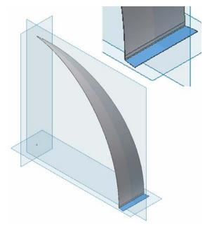
Figure 6A-5A: The inclined end edges of the Bottom Flange of the Gore.
