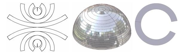
Figure 6A-1C: The poly-conical Method for the approximate development of a spherical surface by substituting the non-developable double-curved spherical surface with segments of developable single-curved conical surfaces. Full spherical surface (left); semi-spherical dome surface (middle); a single conical segment (right).
