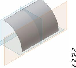
Figure 6A-3E: The Flange Patch Work Plane.
