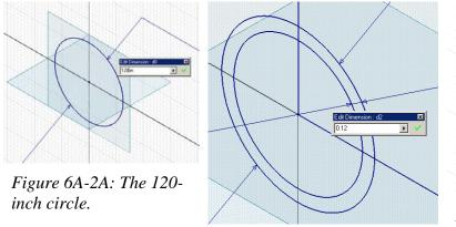
Figure 6A-2B: Offsetting a 0.12-inch circle outwardly.
