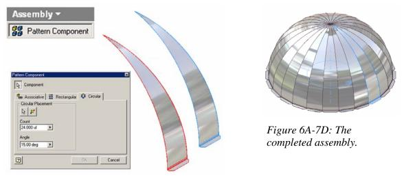
Figure 6A-7C: The Pattern Component tool.
