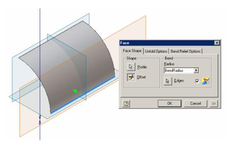
Figure 6A-3H: The direction of the Face extrusion.
