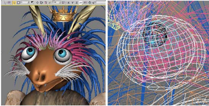
Figure 5-1B: The warped surface of this animal's face is based on polygons that can be considered as further divisible into triangles (created in 3D Studio MAX).
