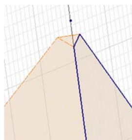
Figure 4B-2D: Projecting the edge lines onto the “ Surface 1 Profile ” sketch.
