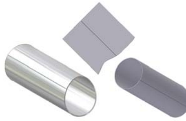
Figure 3A-12D: The intersected cylinder from a plane perpendicular to a slanted axis
