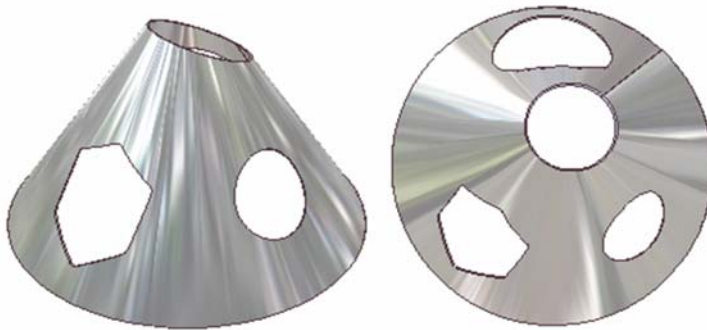
Figure 3A-7F: The cone intersected by the cylinder. The rendered model (bottom).
