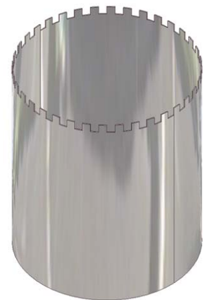
Figure 1G-6E: The folde-up3D model window automatically updating to the assigned material rendering.
