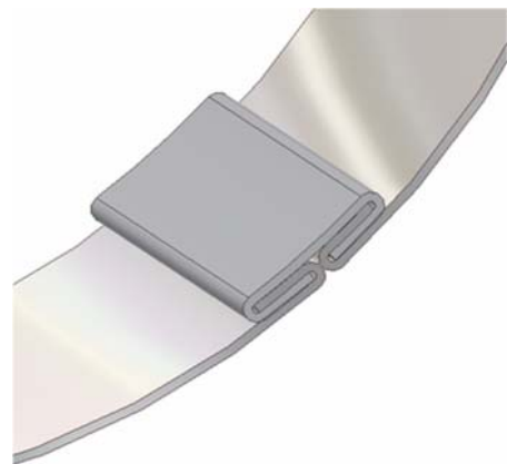
Figure 1F-1A: The cylindrical sheet metal lateral piece with locking seam, created with the Contour Flange tool.
